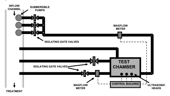
The Facility was originally designed and used by United Utilities for a series of 'in house' long-term CSO Screen evaluations, from which a test procedure known as the "100-Hour Test" was developed. Screens evaluated included the Huber RoK1 Stormscreen' Longwood Stormguard, Kier (now Hydro Int) Heliscreen and the NOV Mono Stormscreen.
